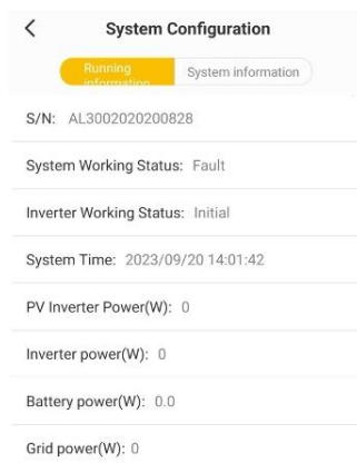
Figure 8-20 Check the power of the photovoltaic inverter
